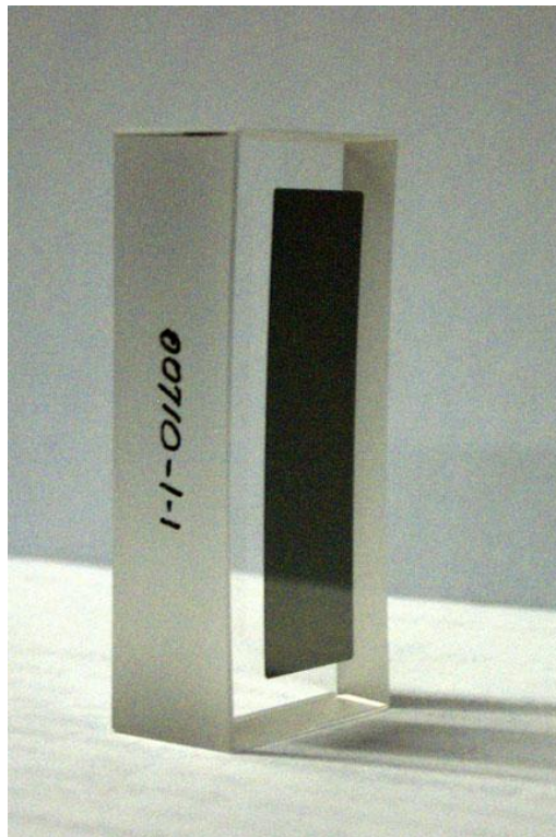
Figure 9. Photograph of an INRAD Germanium Toroid. Crystal cross-section is 12.5 mm x 40 mm.
