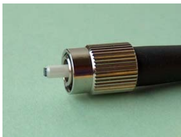
Figure 4.6.2: SAM chip on FC/PC connector end face
