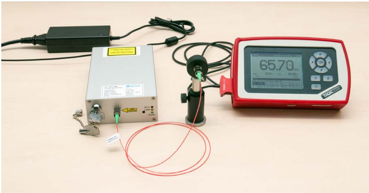
Figure 5.2.1 Setup for measurement of the laser diode LD980 output power as a function of the drive current. The optical power meter is shown on the right side.
