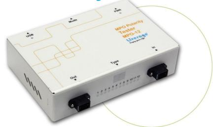
The MPO Polarity Tester is the useful tool designed for checking the defects of a MPO arrayed fiber cable and MPO Connector and identifying the type A/B/C of MPO cable rapidly. The testing works for both SM/MM cable and the MPO Input/output port of PC or APC as well. The MPO emits a visible 650 nm wavelength visible red laser light through fiber optic cables. If there are breaks or defects in the fiber, it will refract the light creating a bright glow around the faulty area.
