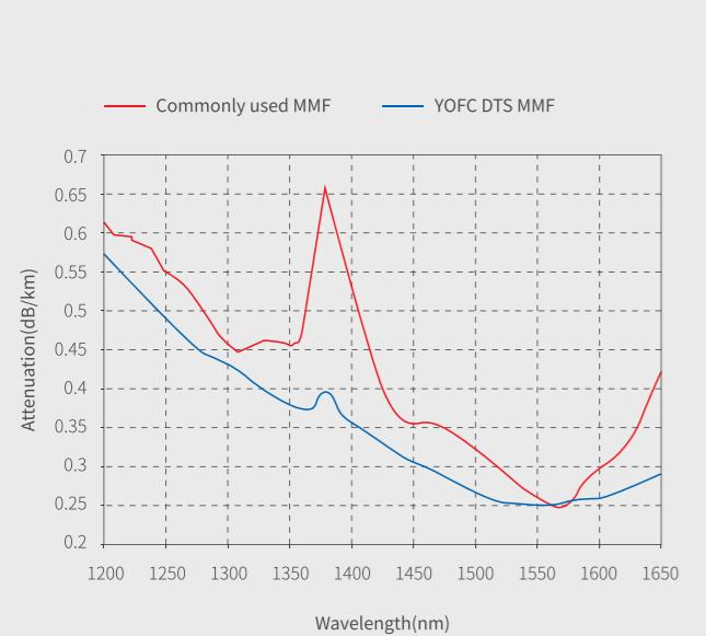
**Compared with communication multimode fibre, the advantages of DTS-MMF are as follows:**
