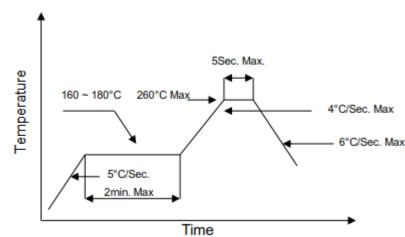
V. SMT Reflow Soldering Curve
