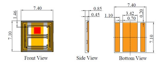
VD-0808I-007W-1F-2A0 with Substrate 6=Cu and Package K=T-mount (unit: mm)
