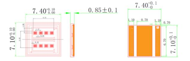
VD-0808I-020W-6K-2A0 with Substrate 4=P/Cu and Package K=T-mount (unit: mm)
