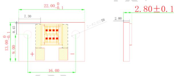
VD-0808I-020W-6K-2A0 with Substrate 1=AIN and Package K=T-mount (unit: mm)
