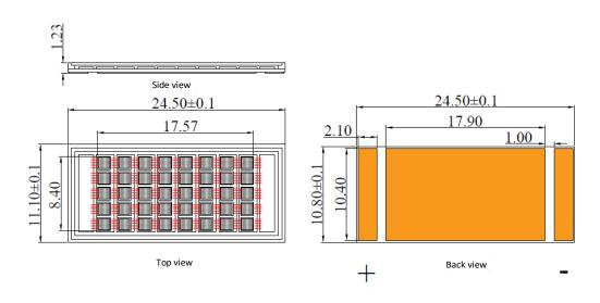
VD-0808I-100W-6K-2A0 with Substrate 6=Cu and Package K= T-mount (unit: mm)
