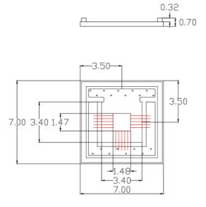
VD-0808P-010W -4K-2A0 (Substrate P/Cu, Package T-Mount)
