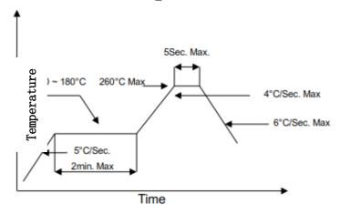
Note: Reflow soldering can be operated only one time. During the temperature ramp-up, no forces may be exerted on the VD which could deform or damage them. After soldering completed, please also do not process until the product temperature ramp down to room temperature.
