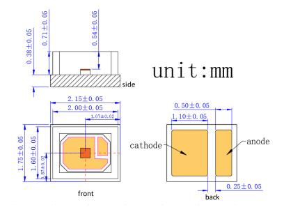
VD-0940V-140M-1C-2B0 with Substrate 1=AIN and Package C=3535 (unit: mm)
