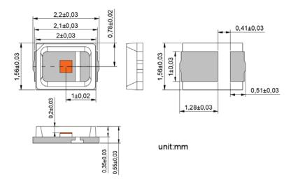
VD-0940V-140M-1A-2B0 with Substrate 1=AIN and Package A=2016 (unit: mm)
