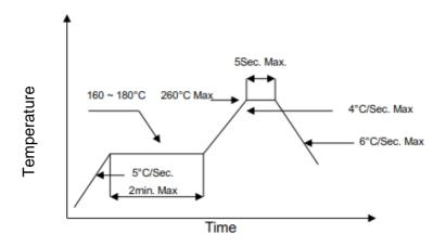
Note: Reflow soldering can be operated only one time. During the temperature ramp-up, no forces may be exerted on the LD which could deform or damage them. After soldering completed, please also do not process until the product temperature ramp down to room temperature.
