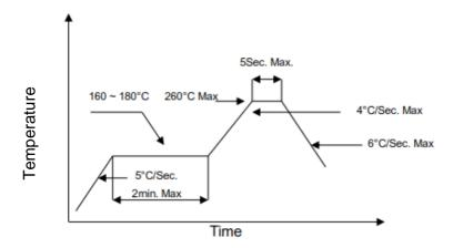
Note: Reflow soldering can be operated only one time. During the temperature ramp-up, no forces may be exerted on the VP which could deform or damage them. After soldering completed, please also do not process until the product temperature ramp down to room temperature.
