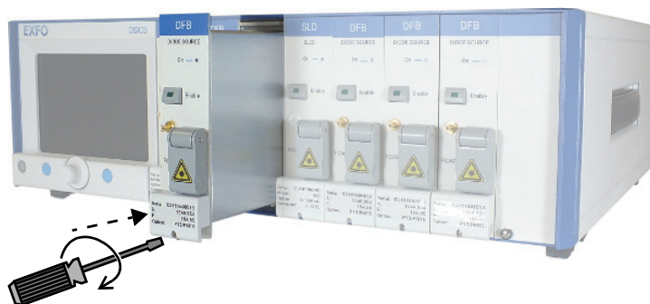
Figure 5: Module Installation – Module Insertion
